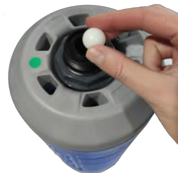
Figure 34: Insertion of ball for air distribution
