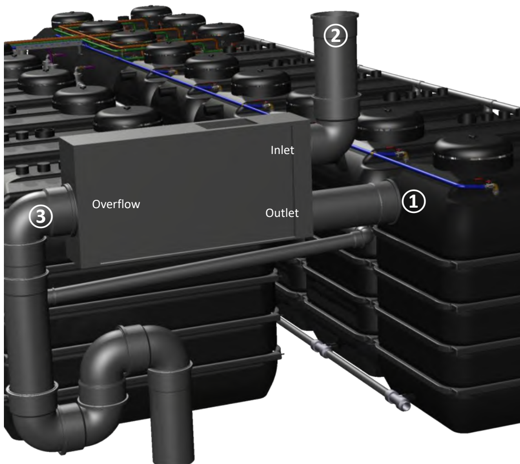
Figure 64: Positioning of the PR300 pre-filter
