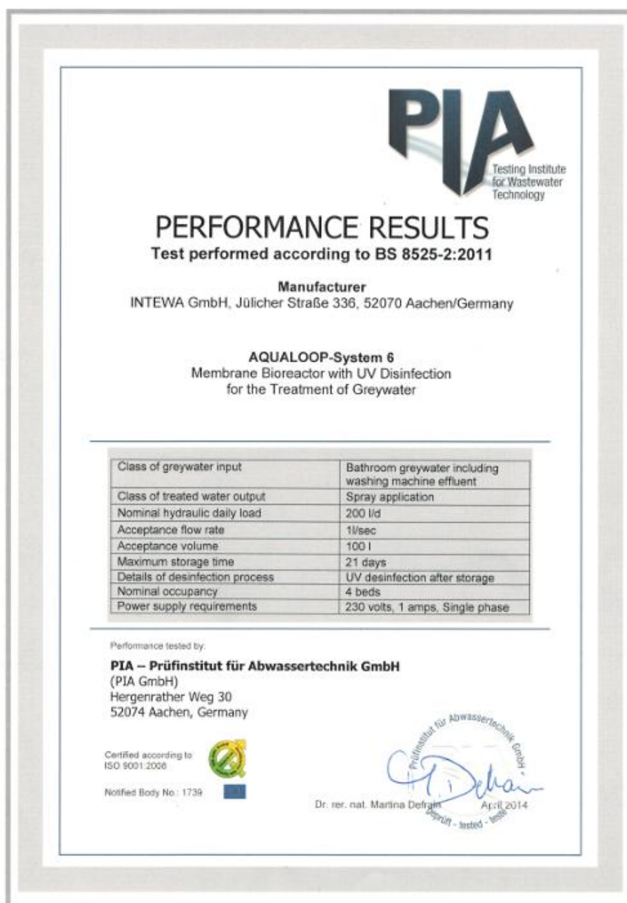
Figure 5: Official test performance results according to BS 8525-2:2011
