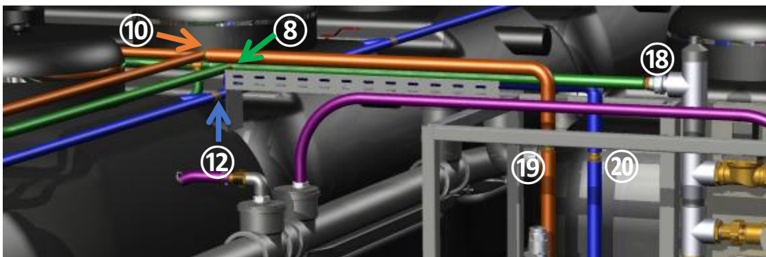
Figure 72: Hose connections between Bioreactor tanks and Technical unit
